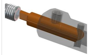
By means of these new tools spanner flats are broached individually. Besides spanner flats with standard wrench sizes also spanner flats with special wrench sizes can be realized without the need for special tools. For each of our MFE-ST broaching tools a range of the width across flats (AF) is stated, which you can adjust flexibly based on your individual requirements. As the tolerance zone of the width across flats can be influenced, the process stability can be increased significantly.
